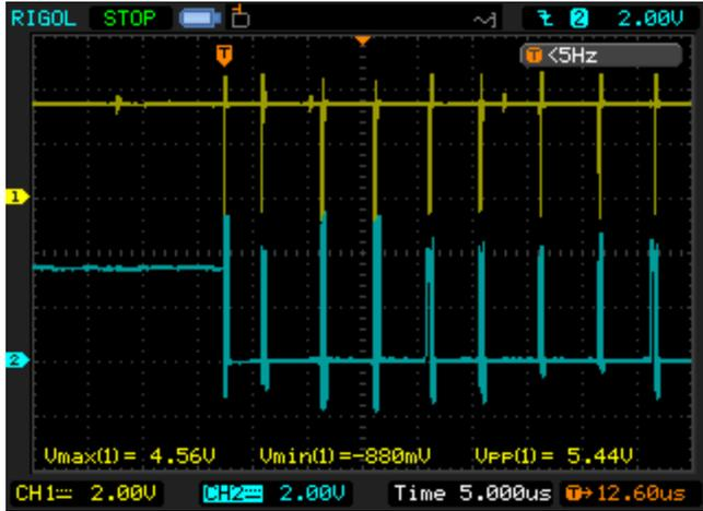
L P C 总线不正常，黄线 L P C F R A M E # 蓝线 A D 1
